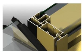
Our louvre mullions have been designed to withstand high wind loads and have a recess on the outside to accept screens when required. The above picture also shows how we fit fixed lights into the louvre frame. This is a clean professional way of making a louvre window next to a fixed light in that the glass is in the same line as the adjustable glass louvre blades.
